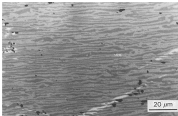
Figure 2 Optical photographs of samples parallel to the growth direction of the directionally solidified \text{Fe}_3\text{O}_4 -YIG eutectic.
